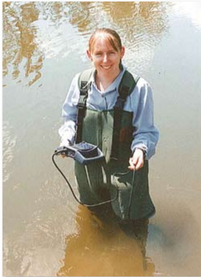
In addition to manual salinity testing (photographed above), approximately 30 automated probes in the Barwon-Darling river system monitor salinity to provide information for improved decision-making to protect town and agricultural supplies and natural ecosystems.
